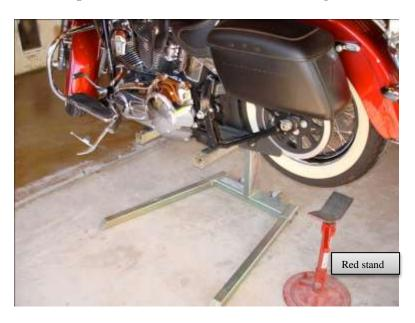
2. Using an 11/16 wrench, remove the forward shock hardware (nut, bushing & cup washer).
