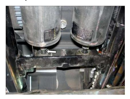
4. Attach a split collar on the shaft of each shock behind the rear bushing cup washer. Use a dab of Blue Thread Locker on the collar bolts.
